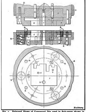
Fig. 3. Enlarged Views of Compound Die used in Sub-press shown in Fig. 2 Similar letters in each case refer to similar parts, but only the
